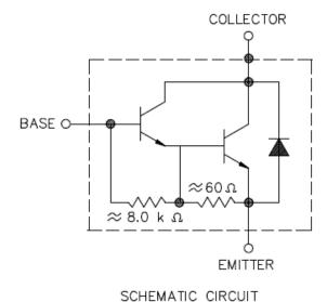
FIGURE 1. Physical dimensions and schematic (TO-213AA, formerly TO-66).
