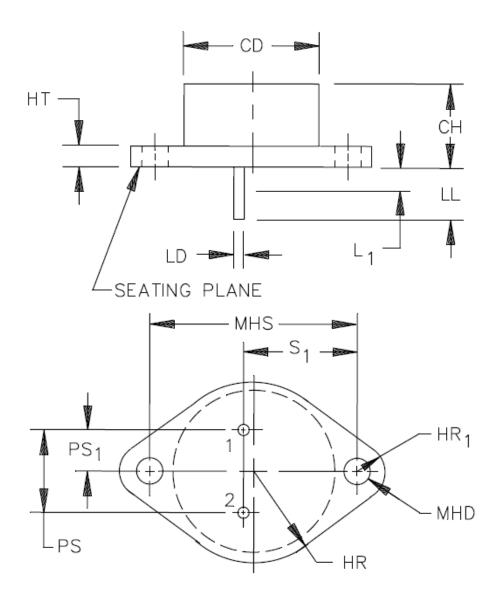
FIGURE 1. Physical dimensions (TO-204AA, similar to TO-3).
