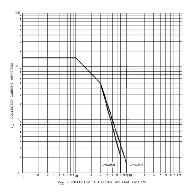
FIGURE 3. Maximum safe operating area graph (continuous dc).
