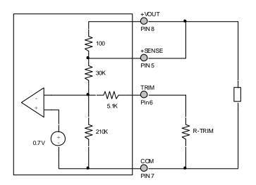
The output voltage is set with an external resistor connected from the TRIM pin to the GND pin 7. This resistor must have a tolerance of 1% or less to achieve an accurate output voltage.
