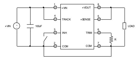
Figure 3 (Shown with recommended 100uF input capacitor)
