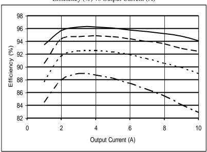
Figure 10 - DVPL0510S Vin=5.0V Efficiency (%) vs. Output Current (A)
