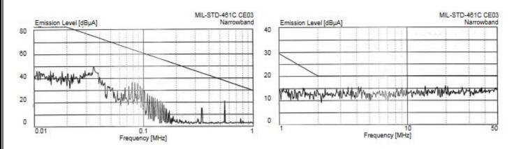
Figure 13- 28V input line, DVME, DVFL and DVPL, C<sub>IN</sub>=100μF
