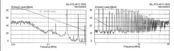
Figure 11 – 5V input line, DVPL, C<sub>IN</sub>=100μF
