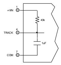
Figure 6 – Internal Inhibit Circuit and Recommended Drive (Shown with optional capacitor for turn-on delay)
